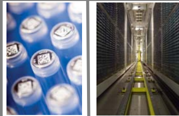
FIGURE 4. UK Biobank utilizes 1 mL Thermo Scientific Abgene tubes (left) linked to unique participant identifier numbers. These tubes are stored in a large automated freezer system (right).
